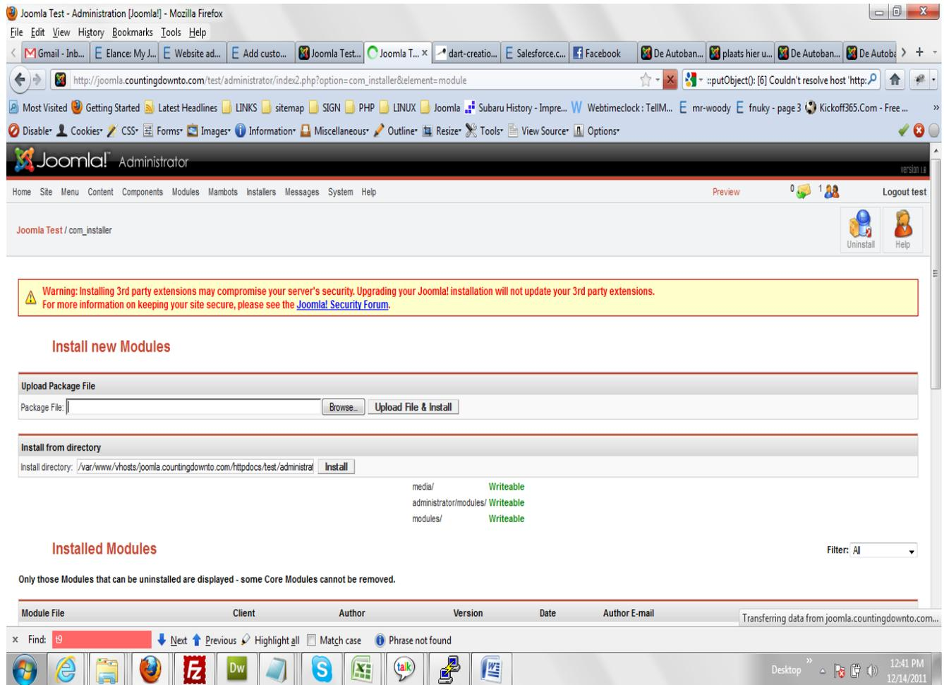
Browse for the module file and click on the upload file & Install. This will install the module.
